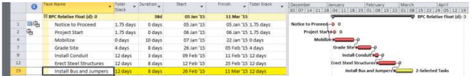
Figure 7: (MSP) BPC Logic Filter - Driving Path to Install Bus and Jumpers
